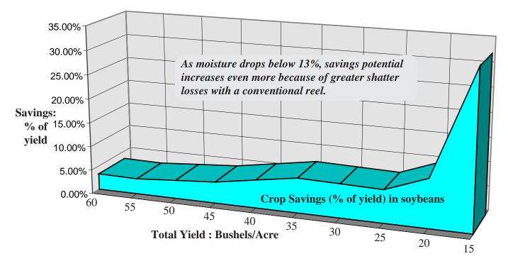
All registered Finger Air Reel Owners who responded to a survey, were averaged into these charts representing their determination of yield savings with the Finger Air Reel vs. a conventional Finger Pick Up Reel in Soybeans.
